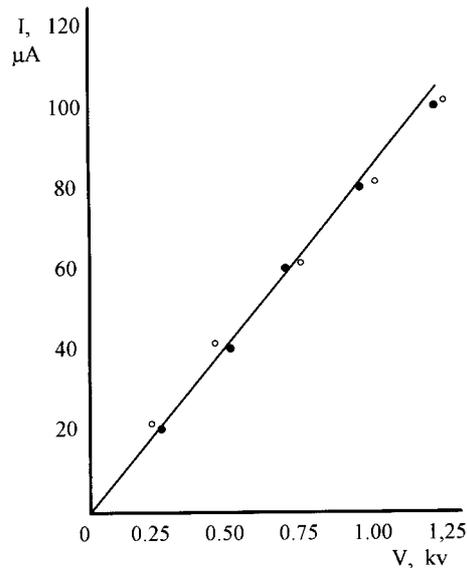
Figure 3: Plot of the output current  $I$  as a function of the voltage  $V$  on the spherical shell. The experimental points are the group average of 15 measurements, the dispersion of which is about 10%. The 2 sets of points (solid and open circles) correspond to 2 independent experimental runs.
