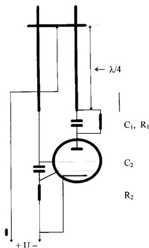
Figure 1: Barkhausen-Kurz's generator. The valve type is 6 $\ni$ 5II. The anode-cathode distance is  $\ell = 0.6$  cm. The voltage  $u$  (see text) is 108 V. The frequency at  $V = 0$  is  $f_0 = 256$  MHz (wavelength  $\lambda_0 = 117$  cm).  $R_1 = 12\text{k}\Omega$ ;  $R_2 = 1.3\text{M}\Omega$ ;  $C_1 = C_2 = 24$  pF.
