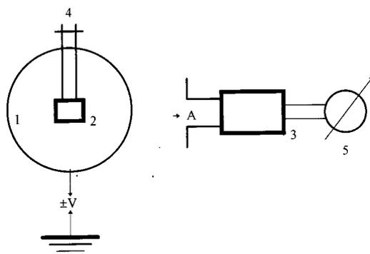
Figure 2: Scheme of the experimental set up : (1) is the spherical shell (it is an In-Ga coated glass sphere) ; (2) is the Barkhausen-Kurz generator ; (3) is the receiver of antenna (A) ; (4) is a quarter-wave resonator ; (5) is a microammeter (output current  $I$ ).
